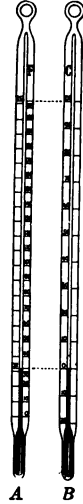
FIG. 30.—Fahrenheit (A) and centigrade (B) thermometers showing the relation of the scales.
